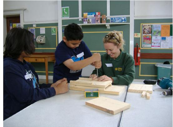
We decided to make the channels for the bats at 20mm and 15mm wide. The 20mm channel width was chosen as it was also the thickness of the wood used, therefore simplifying the cutting. We found the accurate cutting of the channel rails was the most difficult part, given the fact we were using a hand saw and a workmate bench.
